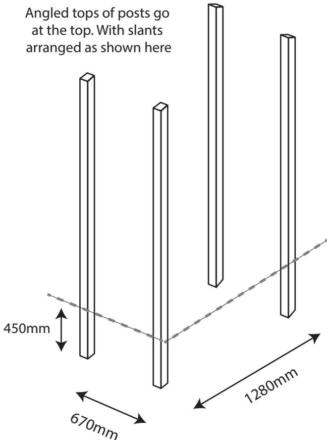
2) Fix trellis between posts approx 75 -100 mm down from top of posts using either 50mm screws if you have English Rose trellis or 75mm screws if you have Square or Heavy Diamond trellis. Fix where indicated with a
