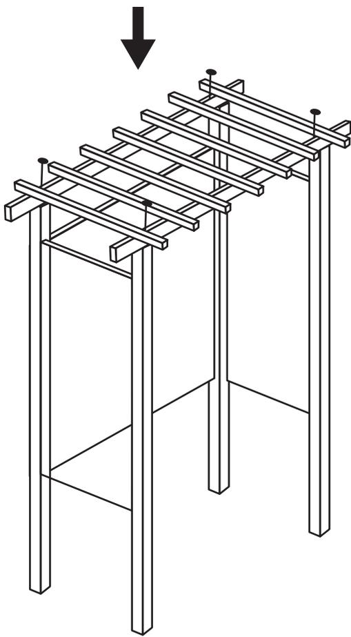
The arbour seat top comes already constructed it is put in place on top of the posts and fixed in using 100mm screws down through the top into the top of the posts where indicated with a
