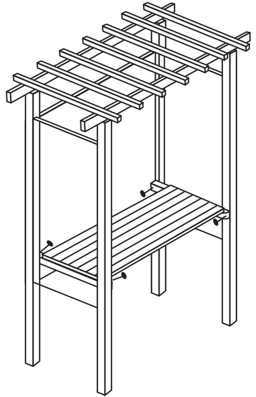
Fix the seat bottom in between posts at desired sitting height. Face fix using 100mm screws where indicated with a
